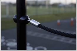
Ropes are made of UV-stabilised PES with inner steel cable reinforcement. The rope is induction treated in order to create a strong connection between steel and rope which leads to good wear resistance.
