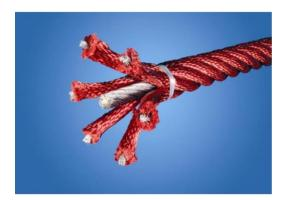
Corocord ropes with 19mm diameter or more are special 'Hercules' - type with galvanised sixstranded steel wires. Each strand is tightly wrapped with PES varn, which is melted onto each indivudual strand. The ropes are highly wear-and vandalism-resistant and can be replaced at site if needed.
