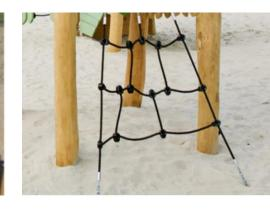
Nets and ropes are made of UV-stabilised PA with inner steel cable reinforcement. The rope is induction treated in order to create a strong connection between steel and rope which leads to good wear resistance.
