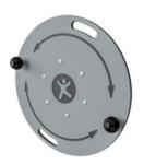
The Ø800x19mm wheel is made from HDPE EcoCore™ plate. EcoCore™ is a highly durable, ecofriendly material, which is not only recyclable after use, but also consists of a core produced from 100% recycled material. The core has a thickness of 15mm and is representing 80% of the total material.
