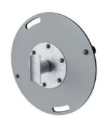
The bearing house is made from hot dip galvanized steel. The bearing shaft is made from stainless steel AlSl304. The bearing itself is made from Polyoxymethylene (POM), an engineering thermoplastic with a high stiffness, low friction, and excellent dimensional stability.
