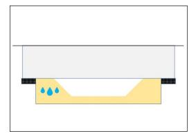
The in-ground galvanized steel frame must be supported with pre-casted concrete blocks/tiles all around the frame. Below the Jumper there must be made an area of drained undersoil to prevent a water puddle. See installation guide for detailed information.
