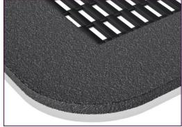
The embedded safety surfacing area around the Jumper is made of EPDM rubber with a thickness of 3 cm. The width of the rubber is 25cm with rounded corners.
