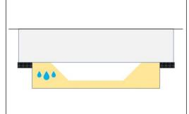
The in-ground galvanized steel frame must be supported with pre-casted concrete blocks/tiles all around the frame. Below the Jumper there must be made an area of drained undersoil to prevent a water puddle. See installation guide for detailed information.
