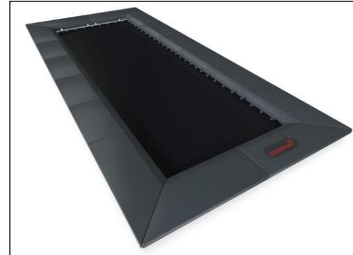
The tiles are molded in grey SBR recycled rubber, Styrene Butadiene Monomer rubber, and the KOMPAN logo is made of EPDM Ethylene Propylene Diene Monomer. Inside each of the rubber tiles there is a 3 mm hot dip galvanized steel plate.
