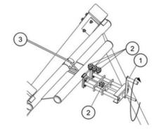
The steel cable 3 is tensioned by a special designed device. By turning the handle 1 the steel cable can be tensioned according to instruction in a safe way. After tensioning the cable is locked by three clamps 2. The tensioning device can also be used for adjustment during annual inspections.
