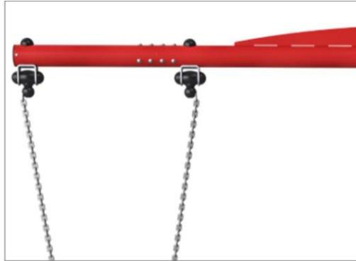
The seat hangers are made of high quality UV-stabilised nylon (PA6) housing with integrated lifetime sealed ball bearings. The chains are fixed by a stainless steel hook with theft proof snake-eye bolt in a turn able anti twist housing.
