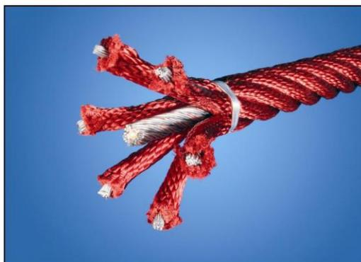
Corocord ropes with 19mm diameter or more are special 'Hercules' - type with galvanised six-stranded steel wires. Each strand is tightly wrapped with PES yarn, which is melted onto each individual strand. The ropes are highly wear-and vandalism-resistant and can be replaced at site if needed.
