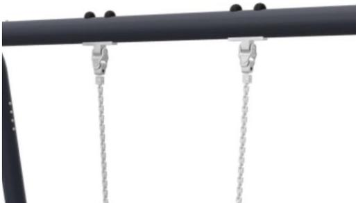
KOMPAN heavy duty designed swing hangers of stainless steel with anti-twist function. The hangers are attached to the cross beam on a welded bracket with two bolts, The bearings are embedded with silicone lubricant and needs no further lubrication.
