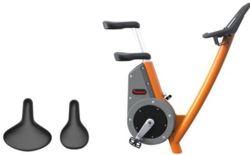
The saddle is made of a Polyurethane Rubber and has a steel insert plate which connects it to the aluminium saddle pin. The saddle can be adjusted to 13 different heights, using a stainless steel pop-pin.
