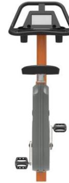
The Q-factor of the bike is 175mm, the crank is made of 18mm stainless steel and connects the pedal arms which are casted stainless steel (grade 304) parts. The length of the pedal arms is 170mm and the pedals are connected with standard bike fittings.
