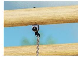
Unique designed swing hangers of stainless steel with anti-twist function. The hangers are attached to the cross beam by a bolt through connection to ensure high durability.
