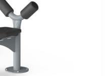
The seat is made of Polyure thane Rubber and has a steel insert plate that is electro-galvanized. The steel plate connects the seat to the frame. This construction makes the seat extremely durable against wear & tear and still very comfortable for a great user experience. The seat is positioned at a height of 46 cm, a comfortable height that makes the transfer from a wheelchair easy.
