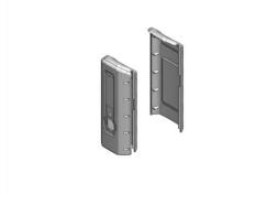
The cover protects all the moving parts from vandalism and entrapments. The cover is made of 5mm rotomolded LLDPE, Linear low-density polyethylene, with excellent impact strength and usable within a large temperature span.
