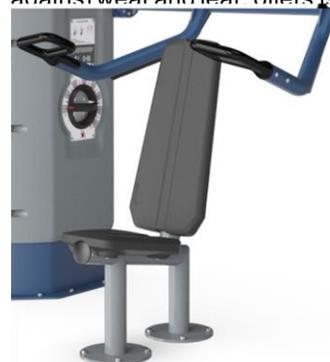
The seat and back support are made of Polyurethane Rubber (PUR) and have an electro-galvanized steel insert plate that connects the seat to the frame. The seat is positioned under a 9-degree angle and the back support has a 15-degree angle. The back support has a groove to relieve the spine, accommodating a comfortable seating position.
