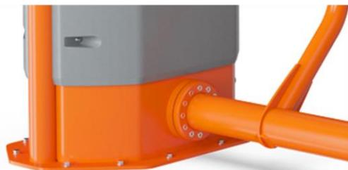
The input shaft is  $\varnothing$ 101,3 x 2,9mm S355 Hot Dip Galvanized and Powder-coated steel. The bearing house is Cast Aluminum (EN AB-44100 / EN AB-41Si2(a)) with self-aligning sealed ball bearings. An extremely strong and durable construction
