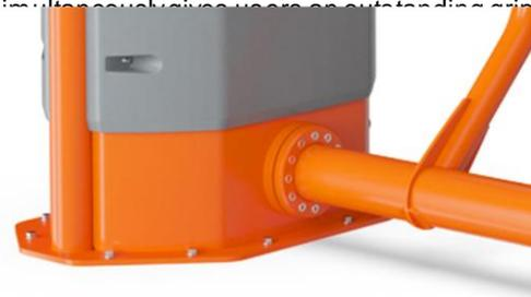
The input shaft is  $\varnothing$ 101,3 x 2,9mm S355 Hot Dip Galvanized and Powder-coated steel. The bearing house is Cast Aluminum (EN AB-44100 / EN AB-ALSi12(a)) with self-aligning sealed ball bearings. An extremely strong and durable construction.
