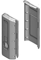
The cover protects all the moving parts from vandalism and entrapments. The cover is made of 5mm rotomolded LLDPE, Linear low-density polyethylene, with excellent impact strength and usable within a large temperature span.
