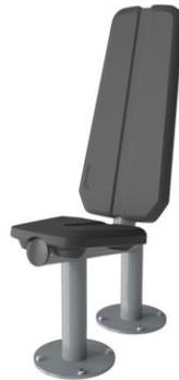
The seat is made of Polyurethane Rubber and has a steel insert plate that is electro-galvanized. The steel plate connects the seat to the frame. This construction makes the seat extremely durable against wear & tear and still very comfortable for a great user experience. The seat is positioned at a height of 46 cm, a comfortable height that makes the transfer from a wheelchair easy.
