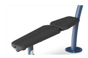
The seat and back support are made of Polyurethane Rubber (PUR) and have an electro-galvanized steel insert plate that connects the seat to the steel frame. The seat and the back support are positioned under an 8degree angle for the correct ergonomics. The back support has a groove to relieve the spine, accommodating a comfortable seating position, another benefit is that it drains water easily.
