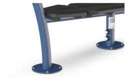
All Steel components are made from carbon steel, with a hot-dip galvanized surface according to ISO1461, and a powder coating corrosion class C3 according to ISO12944-2. Lead content for surfaces is below 90ppm, and below 100ppm for base material.
