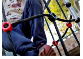
Ropes are made of UV-stabilized PES rope strands with inner steel cable reinforcement. The polyester wrapping is inductively melted onto each strand to obtain excellent wear and tear resistance.
