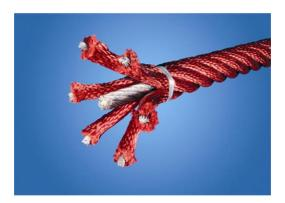
Saturn ropes has six-stranded steel wires and a steel wire core. Each strand is tightly wrapped with PES yarn, which is melted onto each individual strand. After initial friction has removed the surface fibres, a harder PES coating remains to protect each strand, making the ropes highly wear- and vandalism-resistant.
