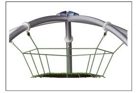
The dome is made curved steel pipes with a diameter of 140mm with hot dip galvanization inside and outside with lead free zinc. Galvanization has excellent corrosion resistance in outside environments and requires low maintenance.
