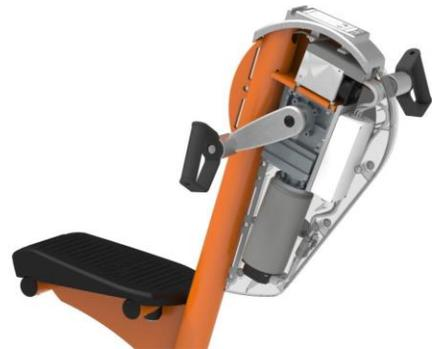
The Innovative self-powered electrical motor and gear providing a virtual flywheel to give real road experience. The resistance works as an automatic drive and adapts automatically to the pedaling speed. The users can overwrite the automatic drive manually by changing the resistance in steps (26 - Watts) through the App.
